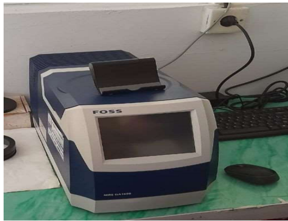
Figure 5.2 Foss NIR DA165 that Owned by PTPN V
